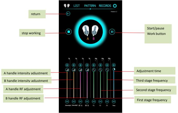
2. Adjust the corresponding intensity/phase frequency/time according to different customer needs. Click the start/pause button to enter the operation work. If the customer requests to pause, you can click the start/pause button to pause the work. After the work is completed, you can directly click the return button to return.
