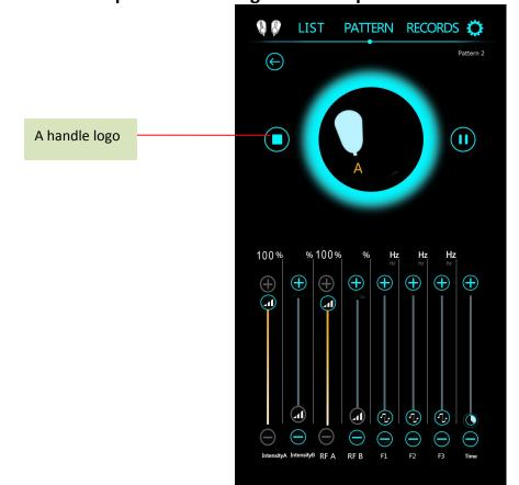
1. The A/B handle can work alone. If you need to stop the B handle when the handle is working, you can click the B handle on the screen (as shown in the figure above, the B handle has stopped working, and the A handle is working again) if you need the B handle Restart work, just light up the B handle logo.
