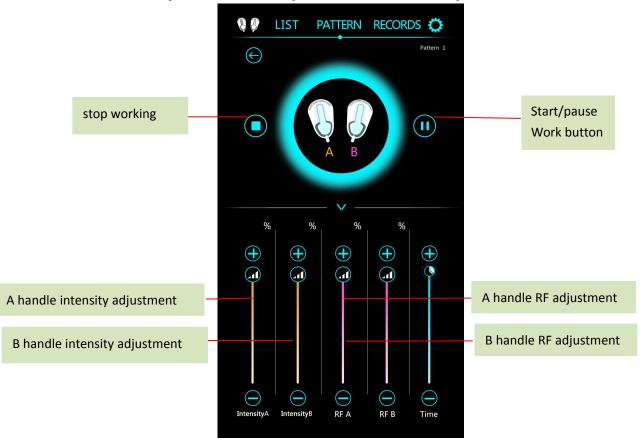
4. Adjust the corresponding intensity according to different customer needs to start the operation. If the customer requests to pause, you can click the start/pause button to pause the work. After the work is completed, you can directly click the return button to return.
